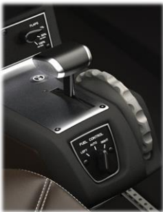
Single lever FADEC Engine Control
